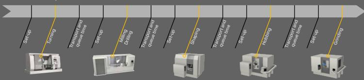
Production line with power skiving | multi-task machine/machining centre + grinding
