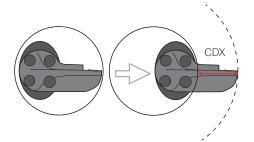
The elliptical shape of the adaptors is optimized for reaching the seat pocket feature. The optimized cutting heads gives you the capacity to reach maximum cutting depth (CDX).
